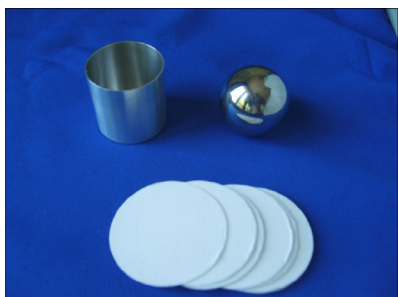
Fig. 2: Set of filters, vessel and calibration ball.
